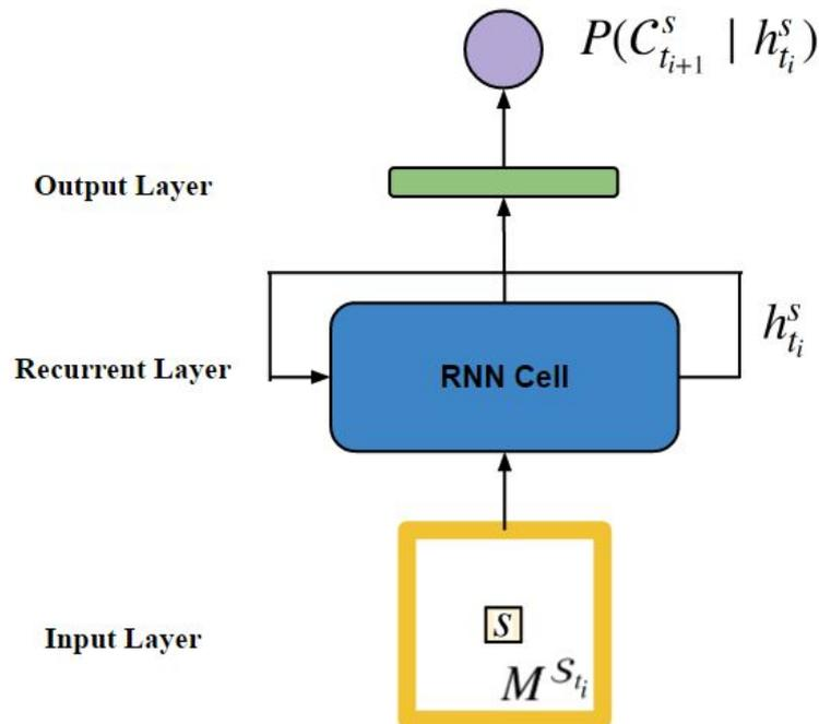
Figure 5. Architect of STNN. For a given sequence  $M^S$ , the recurrent layer learns a representation that summarizes the nonlinear dependency over the previous events. Based on the learned hidden state  $h^S_t$ , it outputs the prediction crime level of cell  $s$  on next time step.
